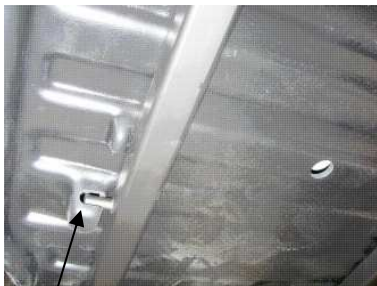
Figure 3.5: Notches and pins at rear of cushion
