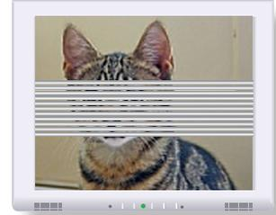
**PROBLEM:** Interference in the form of bars running across the screen while using TV mode.
